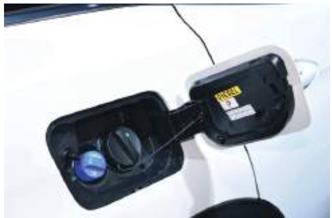
Opening designed for AdBlue® refills in the fuel tank flap - rolled out on all Group vehicles.
